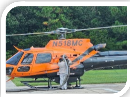
Figure 8. Filling hopper on helicopter with treatment material.
