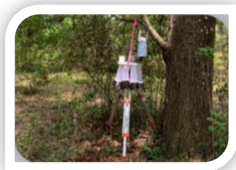
Figure 21. Rotator trap to identify times of peak mosquito flight activity.
