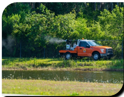
Picture 5: Truck-mounted electric ULV application, photo by Denise Allen, Art You Adore
