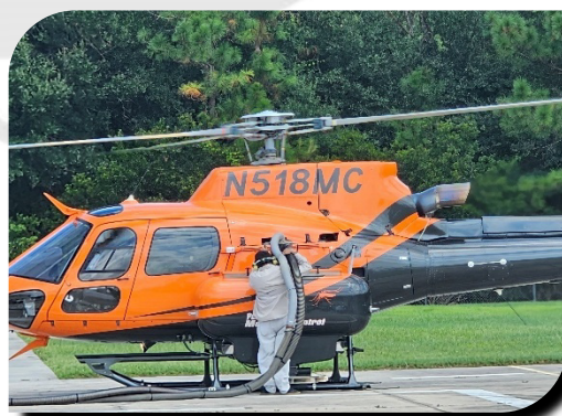
Picture 8: Treatment material filling hopper on helicopter
