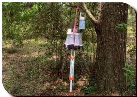
Picture 25: Rotator trap to identify times of peak mosquito flight activity
