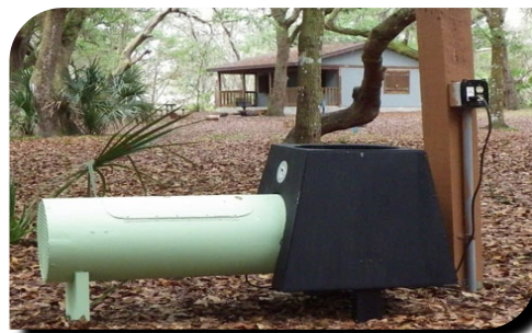
Picture 26: Rotator trap to identify times of peak mosquito flight activity
